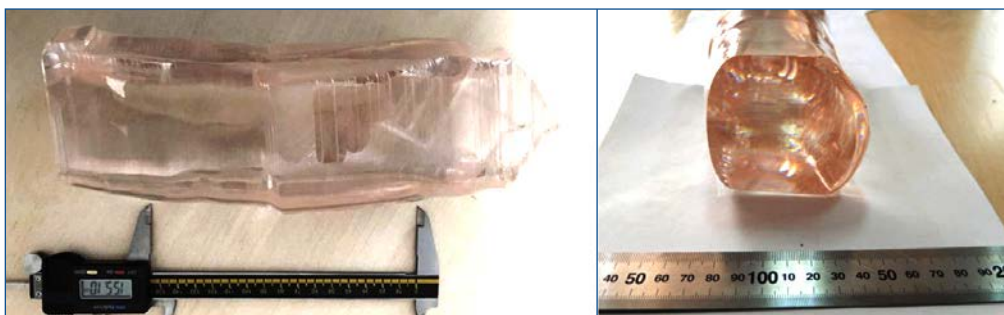
UNIQUE IN WEIGHT AND SIZE SCINTILLATING CRYSTAL \text{ZnWO}_4 GROWN UNDER THE TECHNOLOGY "EXCEPTIONAL ENVIROMENT". Length — 240 mm, diameter — 90 mm
